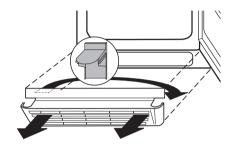
With the door closed, remove the cross-head screws from the lower door hinge bracket and remove the door hinge bracket downwards.
